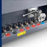
Easily accessible centralized draining system and outlet ball valve
